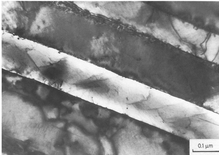
Figure 2 TEM of as-drawn wire B showing subgrains.
