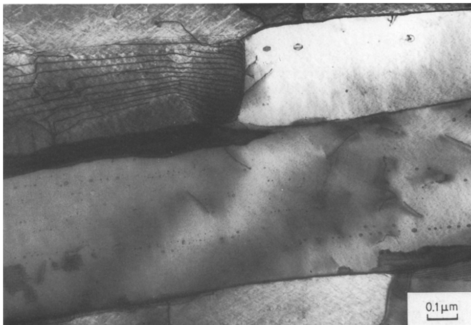
Figure 1 Transmission electron micrograph of wire F after 1 min anneal at 1620°C in hydrogen.
